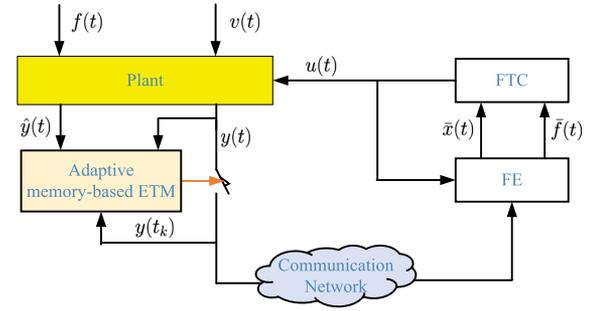
Fig. 1. The framework of the adaptive event-triggered FE-based FTC.
